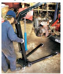
If you're removing or refitting a car engine, this professional quality, hydraulic engine crane is specially designed to fold up for easy transportation.
