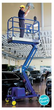
A low level access solution slim enough to fit through a standard doorway yet offering a generous platform height of 3.1m. Ideal for all indoor light repair, maintenance and installation tasks.
