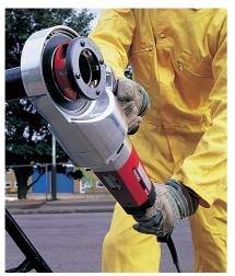
Perfect in tight corners, this hand-held electric threader makes light work of threading mild steel BSP pipes, in situ with pipe clamp or mounted in a pipe vice.
