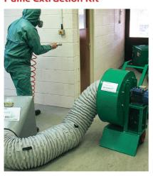
High-volume extraction kit effectively capturing paint, welding, brazing, cutting, exhaust fumes and discharging to atmosphere.
