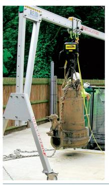
A portable lightweight gantry system available for a variety of lifting applications including confined space, lift shafts, rooftops and clean environments. Its lightweight rigid design and ease of assembly makes it ideal for use on multiple locations.
