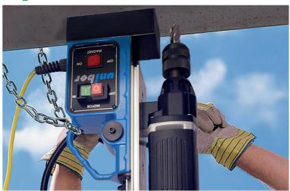
For boring clean and accurate holes in iron and steel, these broachers are ideal for industrial use. A powerful electromagnetic base clamp holds the broacher in place making in-situ work simple. The mini version is ideal for use in awkward locations.
