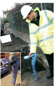
Featuring depth display, left and right indication, current direction and measurement, these precision locators locate and trace buried pipes and cables. They are supplied with a transmitter which applies an external signal for tracing individual pipes and cables.
