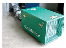
Powerful site dust extractor and filter to cope with large volumes of dust. Designed to give local extraction, air cleaning and to create a negative pressure.
