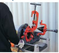
The precision threading of larger pipes up to 4" can be carried out with ease using this threader.
