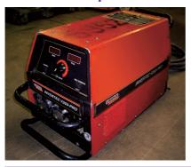
The V350 is a multi voltage power source capable of MMA, TIG and MIG in one small power source. Thermal Arc 300-400amp with SLOPE in and SLOPE out, runs on 415 volts, capable of pulse welding.
