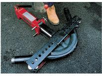
To bend thick-walled steam and gas pipes quickly and easily, these professional benders will provide professional results for pipe sizes between 3/8" to 2".
