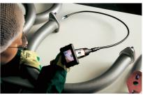
A high-resolution camera sits at the tip of a flexible 900mm cable that is reinforced with a waterproof vinvl jacket. Fully adjustable LEDs offer full lighting control making any inspection job quick and simple.
