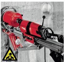
Note: Recommended use of copper washers to ease tightening of cores.
