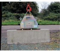
Lift stones, dense concrete and heavy kerbstones with this battery powered stone magnet. It enables quick and easy laying and is capable of lifting stones and concrete up to 400kg.
