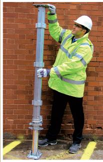
Capable of supporting up to twelve times the load of its steel counterparts, this lightweight aluminium prop is easily handled in awkward locations. The jack has a four start self cleaning threads providing fast height adjustment. Ideally suited for lift shaft applications or back propping of floors.
