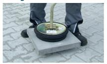
An easy solution to install slabs and paying stones using the vacuum mechanism. This is a good way of laying and moving non porous materials safely avoiding trapped fingers.
