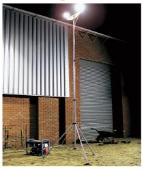
Twin floodlights, mounted on a 6m telescopic tripod mast.
