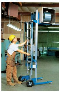
These compact models allow you to manually lift and manoeuvre in congested work areas with ease. With a low loading height of 51mm extending to a maximum height of lift of 3.65m.
