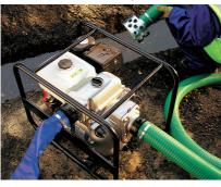
For clearing trenches and deep excavations of water and water-borne debris, this petrol-engine trash pump will handle solids up to 25mm and is capable of shifting over 1300L of water per minute.
