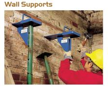
Supporting walls while you fit lintels, RSJs or beams can be tricky. Simply hammer the blade into a raked mortar joint and support it with a steel prop while you remove the masonry beneath.
