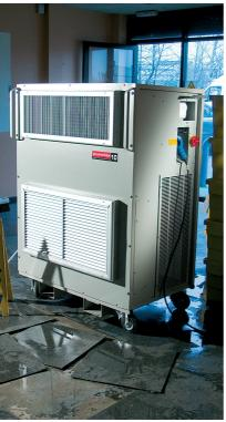
With a maximum extraction capacity of 180 litres a day this unit is our largest dehumidifier. Extracted water can be transferred direct to a drain up to 30m away from the unit which means there is no requirement to empty water tanks. The machine is controlled by thermostat set points.
