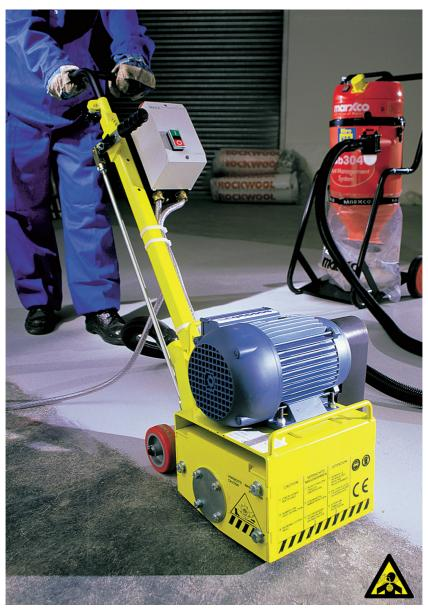
If you are preparing concrete for refinishing, cutting non-slip grooving or removing surface coatings this high-performance scaler gets the job done fast.
