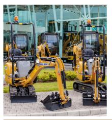
A highly compact unit, which is simple to operate. Able to pass through a doorway and can even be used indoors when fitted with the appropriate exhaust filter.\* Tracks are retractable allowing for easy positioning in tight spaces.
