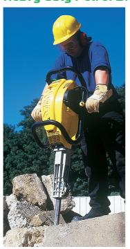
Perfect for emergency work and jobs in awkward locations, this petrol breaker is both portable and lightweight, yet packs the power of a full-sized hydraulic machine. It covers a wide range of applications including breaking concrete, cutting asphalt and tamping ballast, all without the need for power packs and cables
