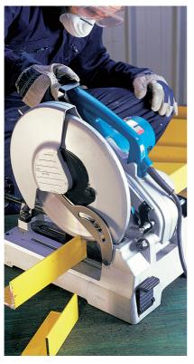
This single speed 300mm TCT Metal Mitre Saw cuts through iron and mild steel with a virtually burr-free, sparkfree finish, making it particularly cost effective in workshop and production environments. With a powerful motor and D-shaped handle for easy gripping the saw will easily cope with multiple mild steel cutting applications from threaded rod and scaffold poles to metal channel. With a maximum cutting capacity of 115mm at 90° and 90mm at 45°, this is an efficient and cost effective choice.
