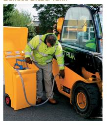
The double-skinned walls of this bunded container make storing and transporting diesel on-site twice as safe. The aluminium hand pump quickly dispenses diesel and is perfect for refuelling generators and other site equipment.
