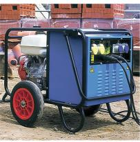
This heavy duty petrol engined unit will generate power for welding mild steel up to 7mm thick.
