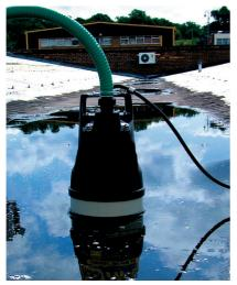
Ideal for pumping out clean water from flooded areas and cellars, this fully submersible electric pump will reduce water levels to within 1mm of the floor.
