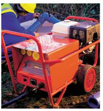
Locating a power source when welding plastic pipes on-site or in remote locations can be a problem. This portable trolley provides the solution by combining our electrofusion pipe welder and petrol generator.
