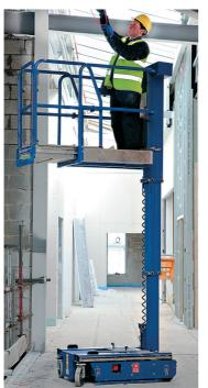
A self-propelled low weight, ultra-compact platform, offering speed and efficiency for many tasks such as light maintenance, inspection and cleaning. The unit has a working height of 4.5m and a low weight of 478kg. This self-propelled unit is rated for indoor or outdoor use.
