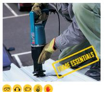
When it comes to cutting sheet materials of all kinds – wood, plastic, metal or plasterboard, this saw can do it. It can also tackle curved as well as straight cuts.
