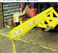
For lifting, moving and positioning heavy loads, these easy to fit attachments turn standard forklifts into mobile cranes in minutes.
