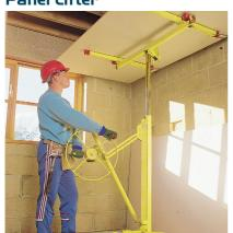
When plasterboarding ceilings or dry lining walls, this lifter ensures it's only a single person job. Lift the panel into position and let the lift hold them while you fix them into place.
