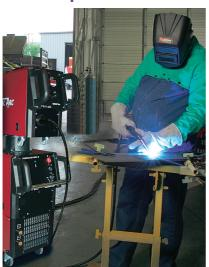
Industrial heavy duty 400amp MIG welding machine with separate wire feeder. This unit will weld up to 1.6mm wire and has a duty cycle of 420amps at 30%. It has digital meters for clear display and timer control. Ideal for semi professional and professional use.
