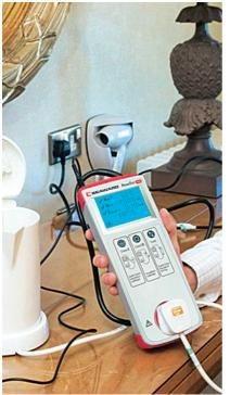
It's a PAT tester, an IEC Lead Tester and a Power Socket Tester all-in-one super compact unit. This product provides everything you need for basic testing facilities. Simply pushing a button will give you the option of either PAT Test mode, Class I and Class II, IEC Lead Test mode or Power Socket mode. This tester is ideal for maintenance staff, schools, colleges, care homes and leisure companies.
