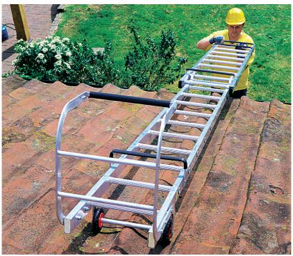
The safe way to reach across sloping roofs for inspection and repairs. Simply wheel these lightweight alloy crawling ladders up the roof and hook them over the roof ridge.
