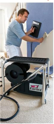
The fast effective way to remove all types of wallpaper, vinyl, woodchip and decorative wallcoverings leaving a clean surface for redecoration, without damaging the plaster. Hold the plate to the surface to soften the wallpaper so it can easily be removed with a scraper in seconds.
