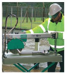
This plunge cut saw bench offers less risk of chipping plus protractor accuracy for complex tile angles. Constant water flow improves blade cooling.
