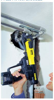
This powerful and portable press fit machine is suitable for producing pipe pressing joints for all common press fitting systems. The standard tool is capable of pressing joints from 10-35mm: It is cordless and well balanced for easy operation/control.
