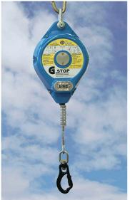
Note: This equipment is designed for use as an arrest/retrieval system. Do not use for raising/lowering of personnel. Lanyards with shock absorbers should not be used with inertia reels.
