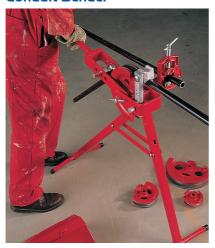
Installing steel conduit runs? Then this specially designed, hand-operated bender will save you time and money by allowing you to produce quick, accurate bends without the need for separate fittings. Handy vice fitted.
