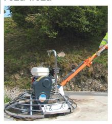
This petrol-driven machine will trowel large, semi-cured concrete areas to a smooth and fine finish.
