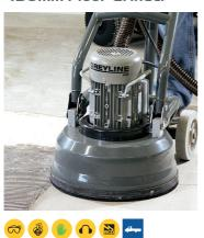
The GL450 is a single phase planetary grinder with three grinding heads and a counter-rotating grinding wheel for a stable grinding without lateral forces. This model of grinder has a larger head for increased planetary performance giving the product a smoother controlled operation increasing productivity.
