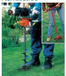
Good post holes are the key to good, long lasting fencing, and here are two borers that will dig them quickly, neatly and with minimum effort.
