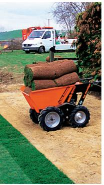
This 1/4 tonne dumper is an exceptional machine for moving building materials and aggregate. This 4-wheel drive power unit is narrow enough to fit through the average doorway for internal work, slip down side alleys or climb over steps and footings.
