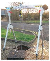
A portable lightweight gantry system available for a variety of lifting applications including, rooftop work with limited access. The very lightweight design and ease of assembly makes it ideal for all goods lifting applications and is also applicable
