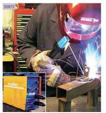
A single-phase inverter for MMA applications with electronic dual voltage facility allowing operation from 110V or 240V. For rods up to 4mm including cellulosic or most other difficult to weld electrodes.
