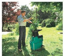
For light garden waste this shredder pulps most organic rubbish down to a mulch for composting.
