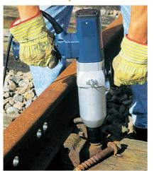
A real labour-saver on vehicle maintenance, fabrication and girder assembly jobs that involve a lot of spanner work. Loosens and tightens large, stubborn nuts and bolts in seconds.
