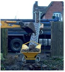
Capable of moving large amounts of waste material, this Shifta Conveyor is ideal for sites where you need to tackle tough inclines with large loads. The open-sided design and V-shaped drive belt moves loads securely without the risk of clogging or unnecessary stoppages.
