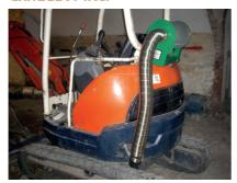
This large exhaust filter is specifically designed for diesel powered plant and machinery to effectively reduce smoke and particulate emmissions. The kit comes complete with a full fixing kit to suit the diameter of exhaust in use.
