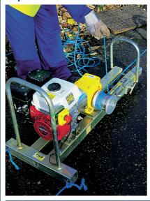
The adjustable frame of this winch is designed for use over most manholes. Lightweight, it will operate anywhere from its own petrol engine.
