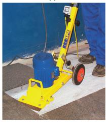
Lifting floor tiles, linoleum or carpet? This easy to use vibrating blade machine will cope with most commercial and domestic surfaces
