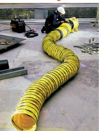
This additional ducting is available for hire with the fume extractor. Both versions come in 6m lengths and can be inter-connected as many times as you require.
