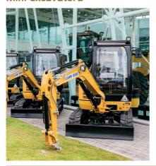
These highly efficient, powerful and easy to operate machines are ideal for many smaller excavating tasks. The modern silenced engines provide operator comfort and are supplied with a choice of buckets, plus a dozer blade. Standard or canopied units are available.
