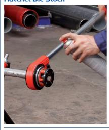
On-site threading of BSP mild steel pipes, whether in-situ or mounted in a pipe vice, is easy with this portable, manual pipe threader.
