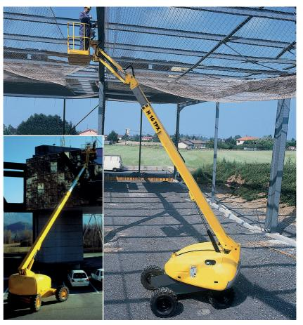
Note: Free site surveys available upon request. These stable and versatile booms can be used in positions from near horizontal to almost vertical on flat, firm surfaces. Working heights of 14-25m can be achieved.
