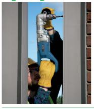
Drilling through joists or in really tight corners? Then you need this specially designed model with its right-angled head.
