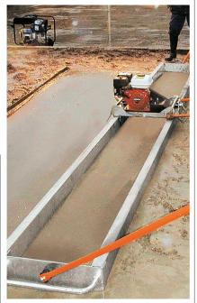
An efficient way to compact and level concrete slabs, rafts and floors, this petrol driven vibrator tackles concrete up to 150mm thick.
