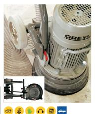
The GL270 is a single headed floor grinder perfectly suited for floor preparation, concrete grinding and surface levelling. This range of grinder effectively removes all types of floor coverings leaving a levelled surface ready to be prepared with a new floor. Also available is the Greyline 270 Edge Grinder, an innovative solution for grinding up against vertical edges.
