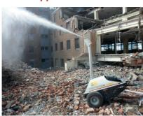
A range of dust suppression equipment units can be supplied in diesel or 3 phase electrical driven options
