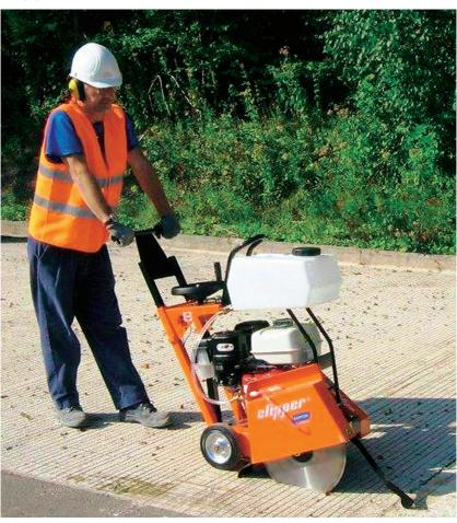
For continuous heavy duty cutting through concrete and masonry pavements, roads or motorways, we have a range of professional floor saws.
