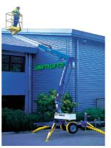
Note: Do not use if windspeed exceeds 28 mph. A range of lightweight electric and bi-energy boom lifts capable of reaching up to a 12m working height. These lifts have excellent reach capabilities and most can be driven whilst fully elevated.
