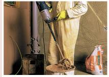
Mixing paints, textured finishes and resins in bulk can sometimes be a real chore but not with this powerful electric mixer. Faster and more efficient than doing the job by hand, it's also ideal for mixing small quantities of plaster.
