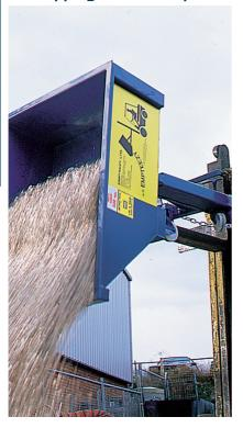
Note: Use correct rated forklift - ensure that the total weight of the skip plus load does not exceed 50% of the forklift rating.
