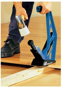
The fast, effective way to lay standard tongue and groove floorboards. Simply position the tool and strike the plunger with the mallet supplied. The efficient ratchet system ensures nails not fully driven by the first blow, remain positively positioned for additional strikes.
