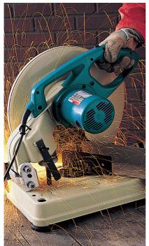
Using a tough 355mm abrasive steel cutting blade and featuring an impressive 115mm depth of cut, this 110V bench top cut-off saw can easily cut metal pipes, rods and sections quickly and accurately on site. The saw has a D-shaped handle for easy, fast and safe operation and an adjustable material clamp for angle cutting.
