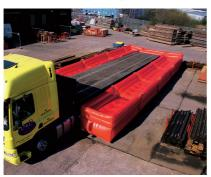
Designed to mitigate the effects of falling from vehicles and trailers. This cost effective fall arrest system comprises eleven inflatable air bags all connected to each other by simple push fit connectors. All can be secured to the vehicle by straps. The mats are then inflated by a 110V electric or petrol motor powered blower.
