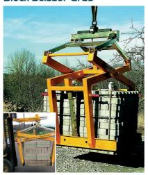
Built to transport vertically steel strapped packs of paver blocks, slabs and kerb stones, this universal scissor grab will safely carry up to 1800kg.
