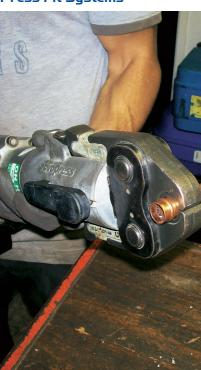
Laois Hire can offer a full range of press fitting systems tools as well as a compliment of jaws and collars up to 108mm. Press fit systems offer numerous advantages including clean, quick installation without the requirement for hot works permits. We have tool solutions for all types of carbon steel, stainless steel and copper press fit systems aswell as multilayer pipe system options including Uponor and Geberit ranges.
