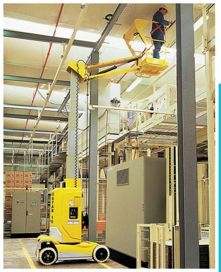
Combining an articulating jib, a tight turning radius and a 10m working height, this machine is the solution for carrying out cleaning, maintenance and repair work in retail stores and factories.
