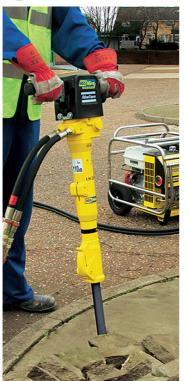
This modern alternative to pneumatic breakers is ideal for asphalt and concrete roads, pavements, paths, patios, drives and slabs. This mobile, heavy-duty breaker combines high performance with low operator fatigue.
