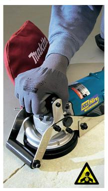
Smooth small areas of stone, masonry and set concrete quickly and easily with this hand-held wheel planer.
