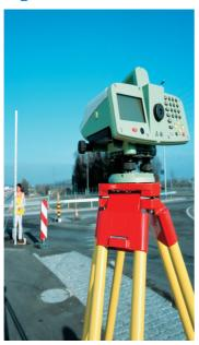
The DNA03 is a digital level with cutting edge technology. The second generation of digital levels by Leica with modern and ergonomic design, large Ic display and excellent optical and mechanical systems.
